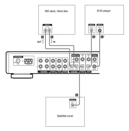
\* Connect to either the COAX IN or the OPT IN jack. We recommend making connections to the COAX IN jack.
